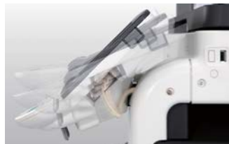
Tilt the screen vertically by 22° in 3-step increments and 15° horizontally.
